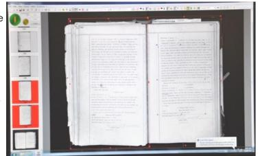
Quality Targets permit operators to view image quality at the time of the scan. Images, even with scanning on different devices, are "normalized" as if they were from the same scanner. Rather than using ad-hoc algorithms and tricks, this software measures image quality and propagates this data through the imaging chain. The Quality Targets establish the baseline digital capture quality of the scanner at the time of scanning.
